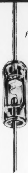
Fig. 1. The "whisker wire" in this 1/4" long, glass-encased diode is bonded to the semi-conductor forming a gold-germanium eutectic alloy at the junction.
